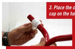
3. Place the cover cap on the handlebar.
